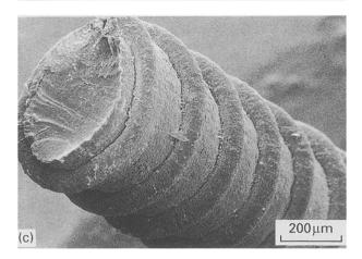
Figure 1 SEM micrographs of as-spun fibres obtained from solution of 5 g/dl (a), 7 g/dl (b) and 12 g/dl (c), and broken in liquid nitrogen.
