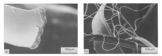
Figure 4. SEM micrographs of fracture surfaces of solution spun PLLA fibres drawn at 200 °C with a draw ratio of 6 (a) and 12.4 (b).
