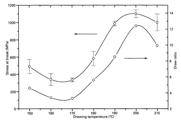
Figure 2 Stress at break and draw ratio of solution spun fibres as a function of drawing temperature.
