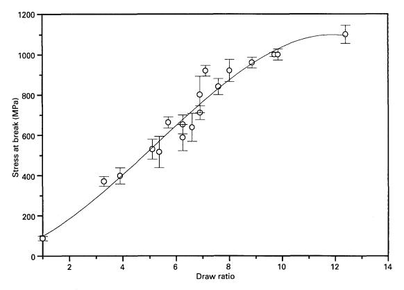
Figure 3 Effect of draw ratio on stress-at-break of solution spun fibres collected at a winding speed of 2 m/min and drawn at 200 °C.
